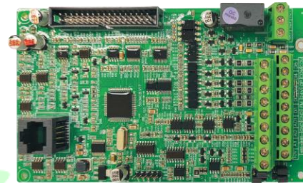
Figure 3-8-1 Terminal layout of 600SCB series control circuit (This control board is an optional product)
